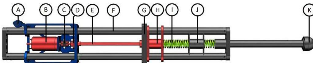
Leg design with encoder for the leg length (A), motor for linear actuation (B), coupling (C), ball screw bearing (D), ball screw (E), tubes for linear guidance (F), end stop with damping for the spring (G), ball screw nut (H), spring (I), buckling preventer (J), spherical foot (K). The hip part (blue) and the linear actuator (red) features 4 PTFE slide bearings and slide freely over the tubes (grey).
